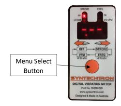
3. Once the equipment is in operational the DVM will change to read stroke amplitude as shown below.
