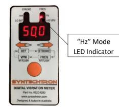
Press the button again to switch DVM to display the frequency in which the equipment is operating in Vibrations Per Minute (VPM) as shown below. Multiply displayed number by 10.
